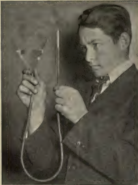
FIG. 1. The water in the tube rises to the level of the water in the funnel.
